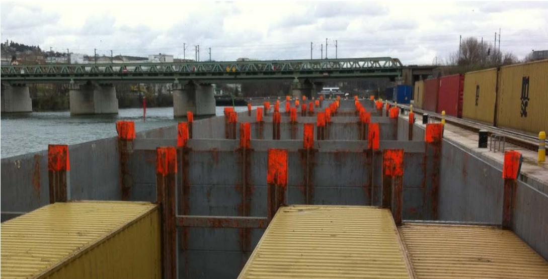
21. Container vessels are often loaded with a considerable gap between container rows. This applies, for example, to vessels that are not quite capable of accommodating three rows of containers side-by-side. Please note, however, that if the gap is too big, the containers can shift in the event of heeling, shocks or collisions. Where appropriate, ensure there is no gap between containers.
